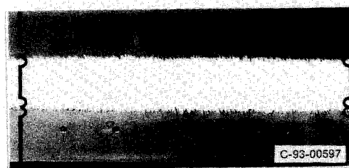
Fig. 8 Severely damaged braided ceramic rope seal (center portion shown) after a hot-scrubbing test demonstrating the need for rub-tolerant seals.
