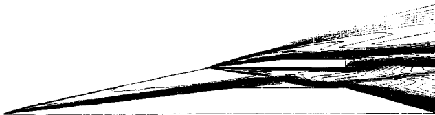
Fig. 18 Mach number contours, laminar, M = 10.1 .
