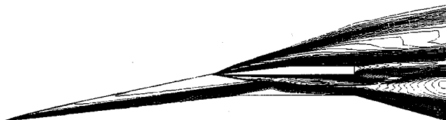
Fig. 13 Mach number contours, laminar, 265 \times 215 , M = 12 .
