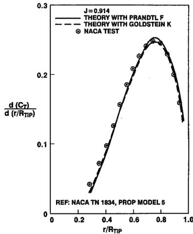
Fig. 10 Comparison of propeller analyses thrust coefficient.
