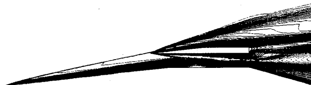
Fig. 14 Mach number contours, turbulent, 265 \times 215 , M = 12 .
