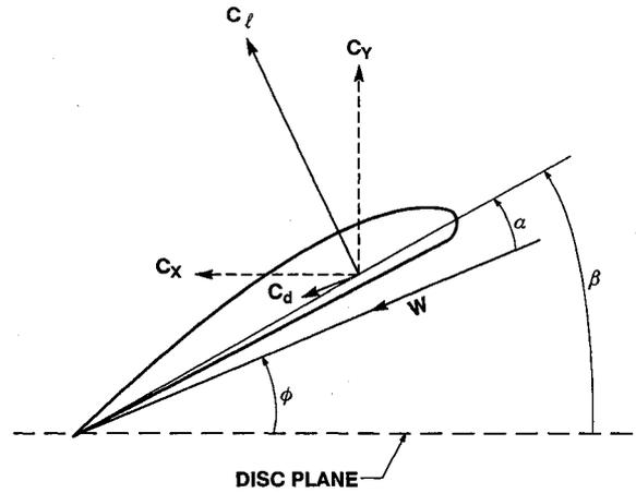
Fig. 4 Force coefficients for propeller blade element analysis.
