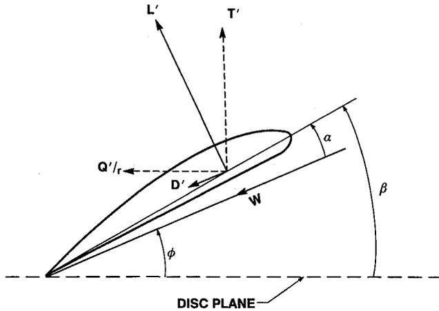
Fig. 3 Force diagram for a blade element.
