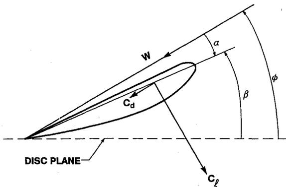
**Fig. 6 Force coefficients for windmill blade element.**
