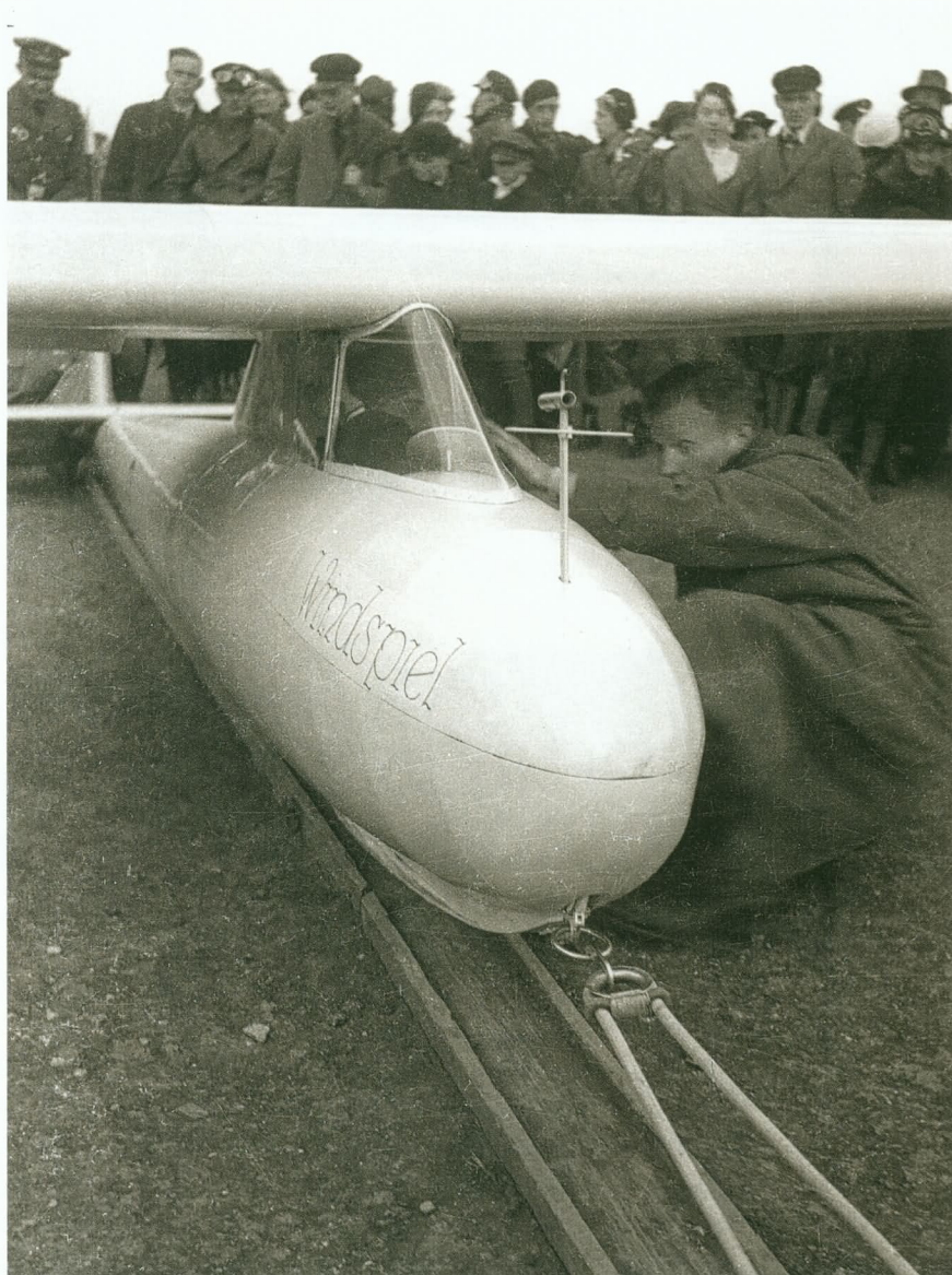
Windspiel ready for launching. The horizontal bar on the mast gave the pilot a guide to the trim attitude
