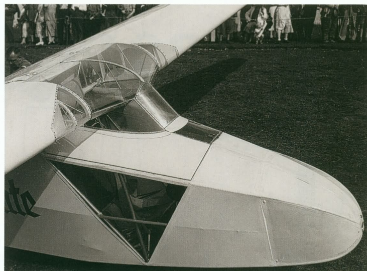
Above: Cockpit canopy and transparencies of the Atalante.
