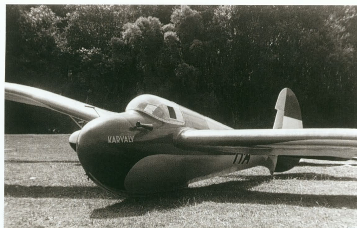
Right above: The M - 22 had a variety of cockpit canopies, some fully moulded in plastic.
