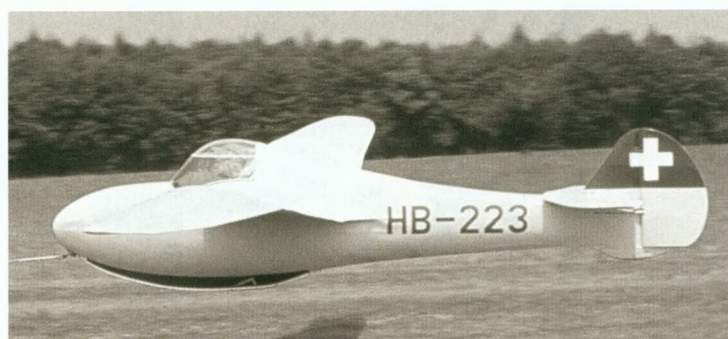
Below: The wing roots gave the pilot elbow room.
