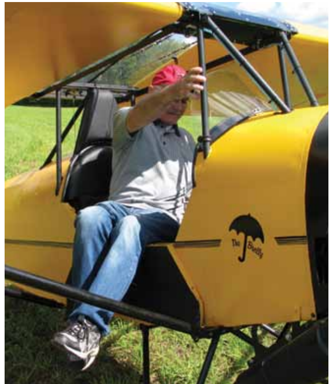
Cockpit access is improved with the optional drop-down door. Jimmy also removed the X-wires between the lift struts and substituted drag-antidrag bracing inside the wings. The Parasol owes a lot to the venerable Baby Ace
