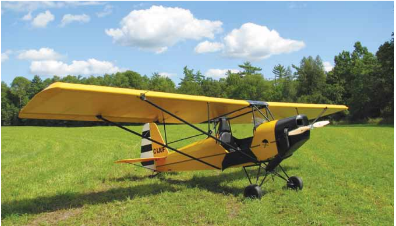
Cockpit access is improved with the optional drop-down door. Jimmy also removed the X-wires between the lift struts and substituted drag-antidrag bracing inside the wings. The Parasol owes a lot to the venerable Baby Ace
