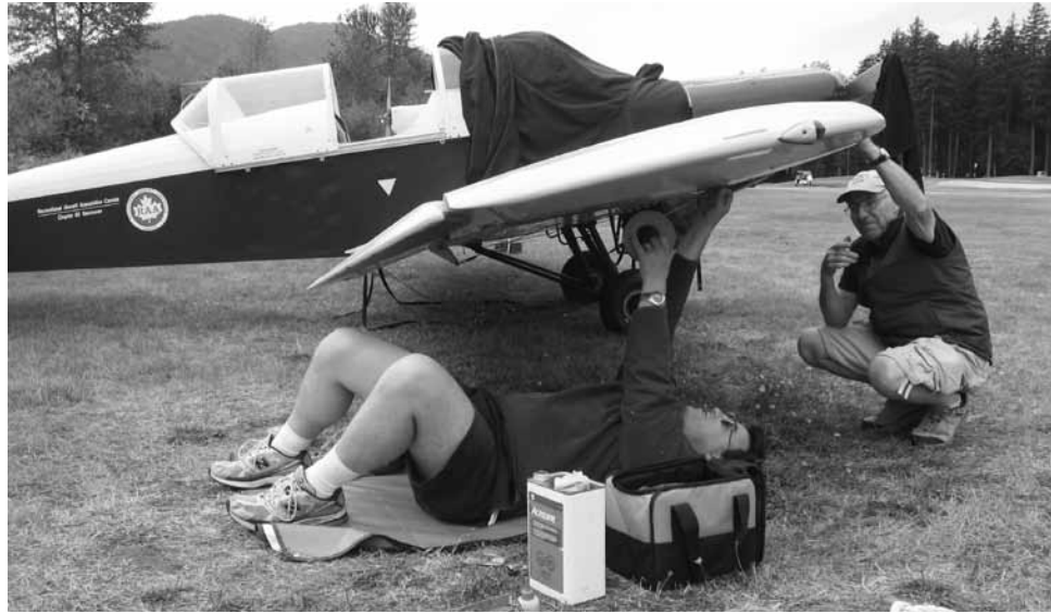
Chapter 85 members Mark ter Keurs and Paul Trudel performing a field repair on the Turbi. Its wing had been damaged by a poorly marked signage the aircraft taxied at a Fraser Valley grass strip. It was assessed safe for a ferry flight after field repairs and returned to Delta Airpark where it is undergoing the full treatment.
