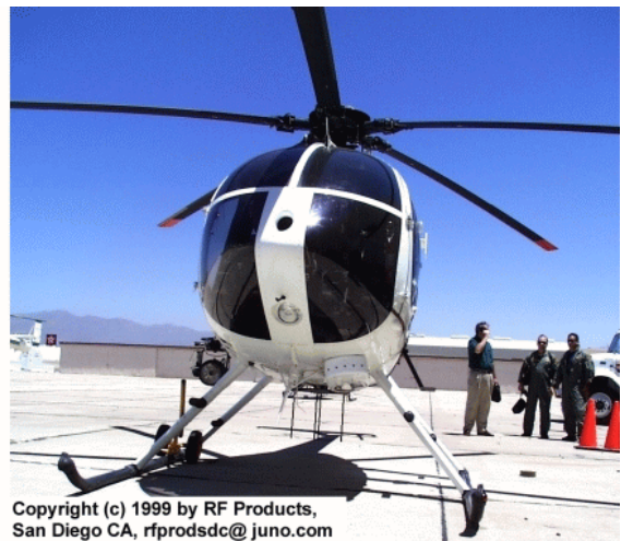
Figure 10 - VHF DF Antenna Mounted On Search-And-Rescue Helicopter
