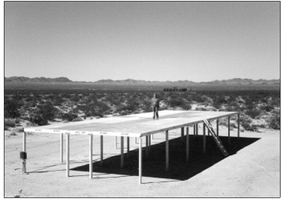
Figure 9 - RDF Products 20' x 60' Elevated DF Antenna Test Range
