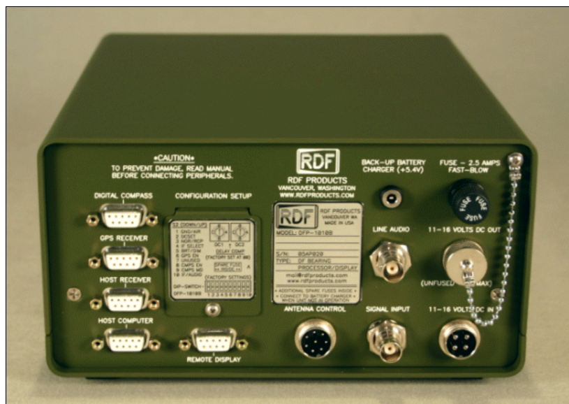
Figure 4 - DFP-1010B RS-232 DF Bearing Processor
