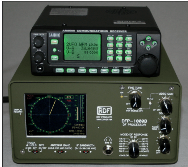
Figure 5 - DFR-1000B Wideband VHF/UHF DF Receiver
